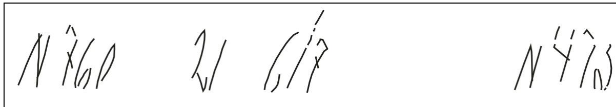
Fig.4 Signs from the collar beam later added to the construction in the roof frame of St Jacobs Church in Tarchomin, Warsaw
