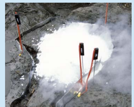
Fig 36 The hurdle is isolated and \text{CO}_2 pellets are being applied. Thermocouples are inserted around the hurdle.
