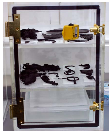
Fig 58 Controlled air drying using saturated salt solutions.
