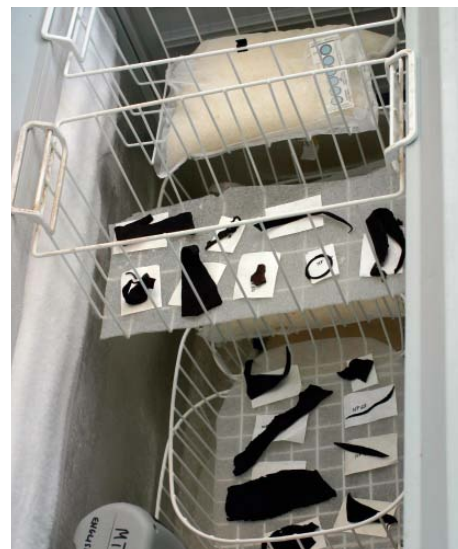
Fig 57 Non-vacuum freeze drying in a domestic chest freezer.
